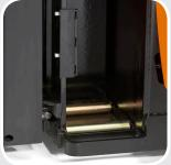
3. The design of the battery compartement allows easy access for maintenance purposes. The battery is mounted on rollers, which enables quick changing of the battery and supports multi-shift working.
