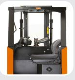
2. New comfortable seat and ergonomic driving position. The b2 control panel has a completely new digital display and control buttons in the middle.
